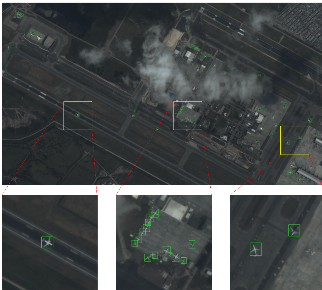
Fig.2. The samples of detection results, the green rectangle denote the detection windows generated by our method. Each of yellow rectangles represents a 300 \times 300 region.
