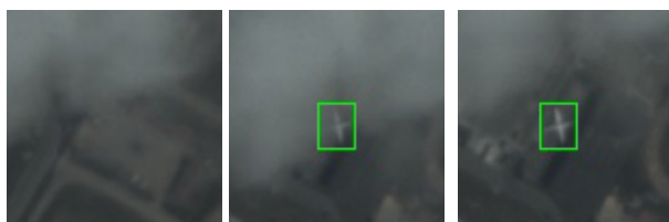
Fig.3. The detection and tracking results of 30-th, 50-th and 70-th frames for object covered by cloud. The size of each image cropped from the frame is 100 \times 100 .
