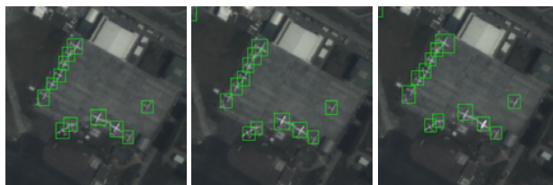
Fig.4. The detection and tracking results of 30-th, 50-th and 70-th frames for static objects. The size of each image cropped from the frame is 300 \times 300 .
