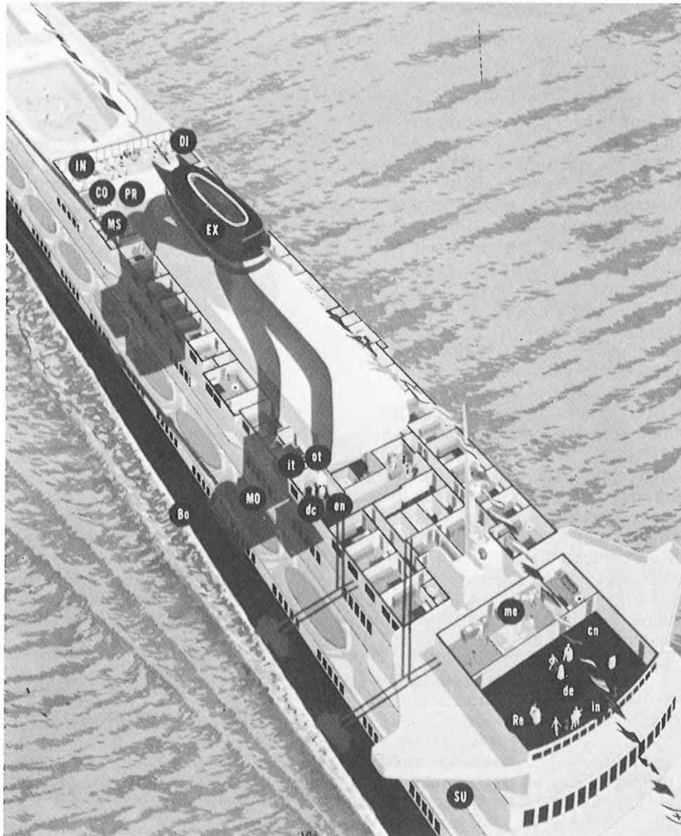
Figure 2.2(b): Major subsystems for an ocean liner
