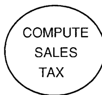
Figure 9.2(a): An example of a process
