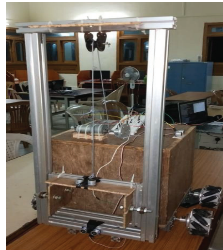
Fig. 10. Prototype of Autonomous wall painting robot
